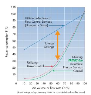
Energy savings can be achieved by utilizing variable speed drives to reduce the motor speed for meeting demand flow in place of mechanical flow control devices, such as dampers or valves. The Affinity Laws for centrifugal loads state that flow is proportional to motor speed, pressure is proportional to motor speed squared, and power required is proportional to motor speed cubed.
